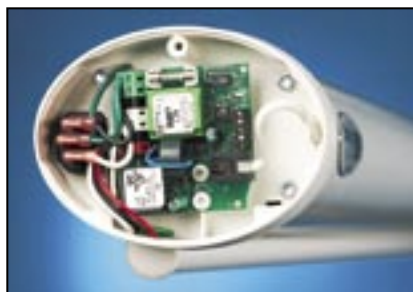
Built-in controller and IR receiver
